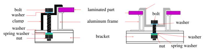
Figure5 Clamp installation guideline
