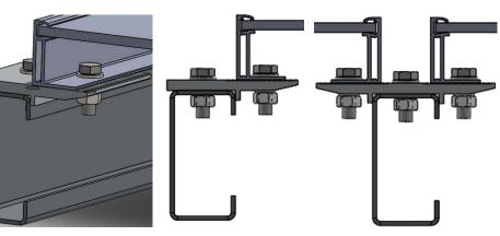
**Figure 7 Installation Mode**
