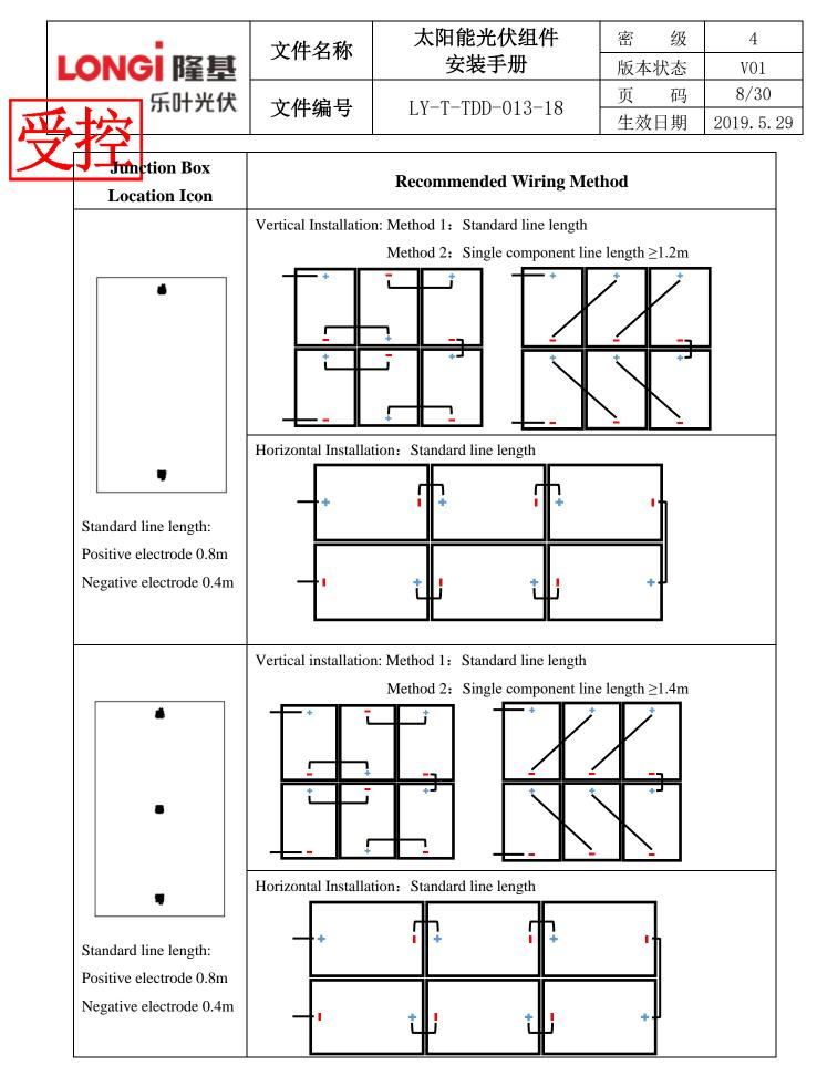
Figure 3 Junction Box Style and Wiring Method
